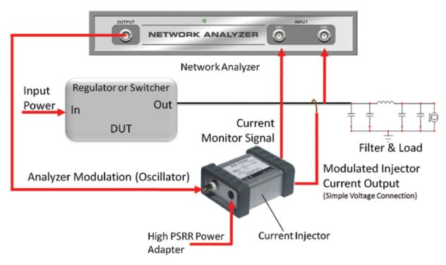
The J2111A Current Injector supports Non-invasive phase margin measurements. You can actually use it to measure the stability of your power supplies WITHOUT having to break the control loop. Simply connect the Current injector output (+ and – leads) to the signal of interest and you can measure the impedance, stability, or step load response.
