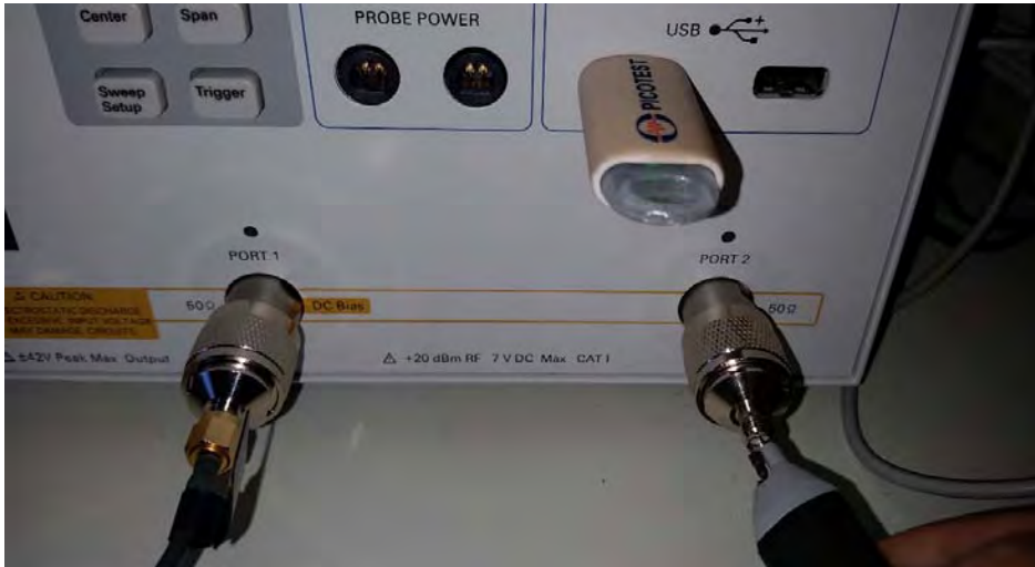
Figure 12: The S-parameters of 1 port probe, S11, S22 and S21, are tested using the E5061B VNA. The CH2 terminator is used as the MATCH load.
