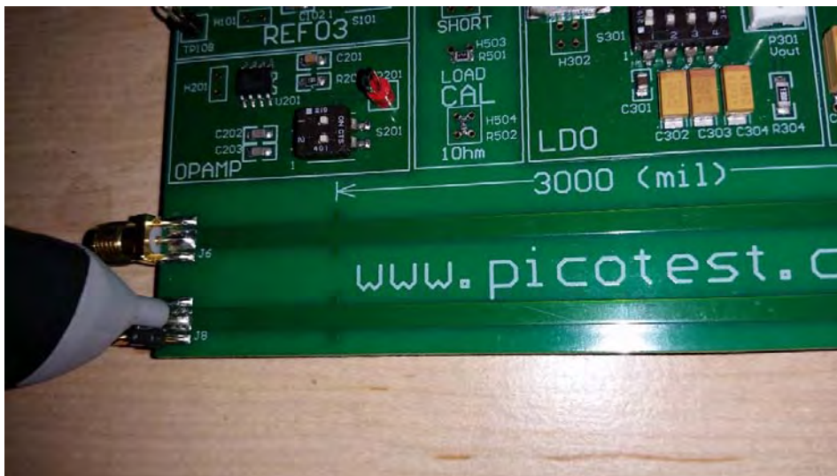
Figure 18: The 1-Port probe is used for TDR measurement on the VRTS3 test board.
