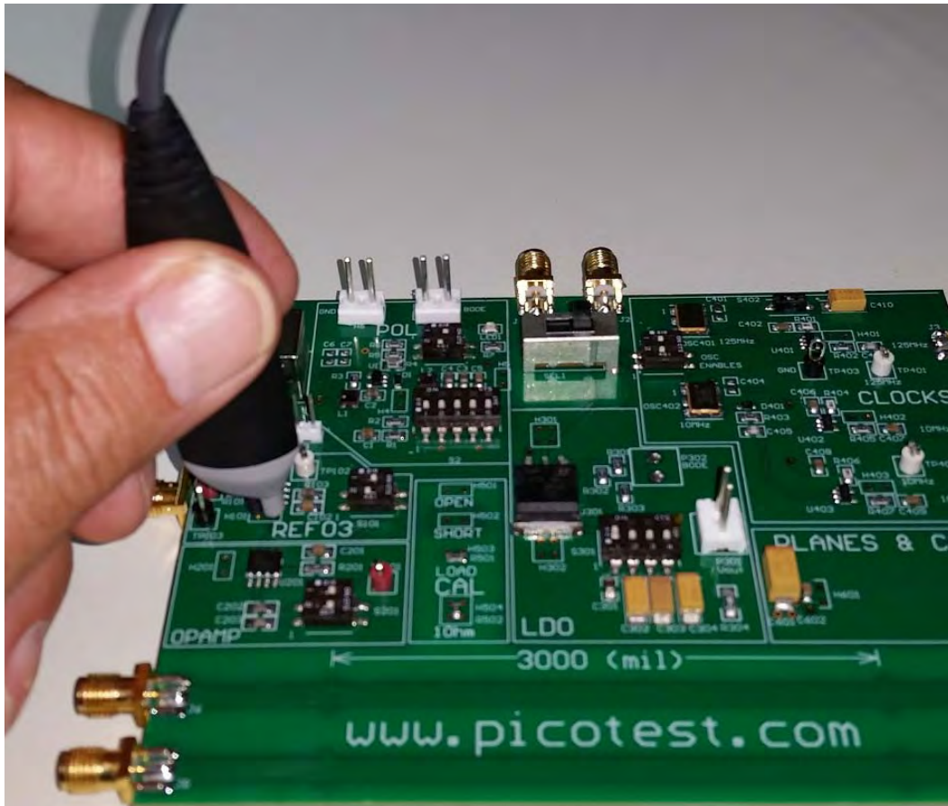
Figure 16: 1-port probe connected to H101 to measure the impedance of a voltage reference. This same test can be performed on any power supply control loop including those of POLs, switchers and linear regulators.
