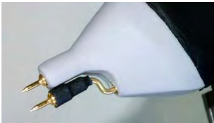
Figure 3: Probe head. The 1-Port probe on the left shows the stationary tip and swiveling/replaceable ground lead. The 2-Port probe on the right shows the 2 ports connected forked 2 prong probe tip and hole for the ground lead (no ground lead connected).
