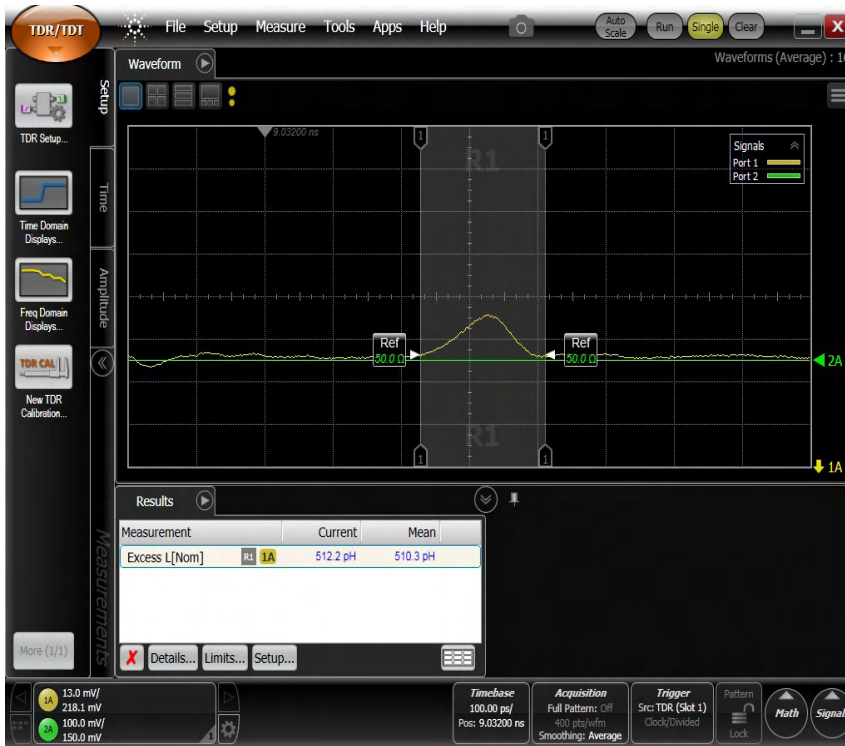
Figure 19: The excess inductance resulting from the hole in the ground plane.
