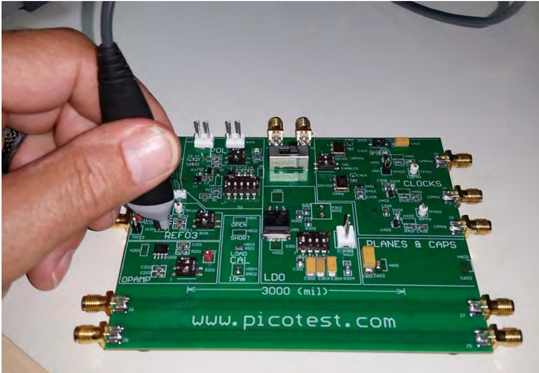
Figure 5: Making a measurement with the 1-Port probe. It is often necessary to set the ground pin placement first using the variable pitch pin and then apply the signal pin connection, rotating the probe into place.
