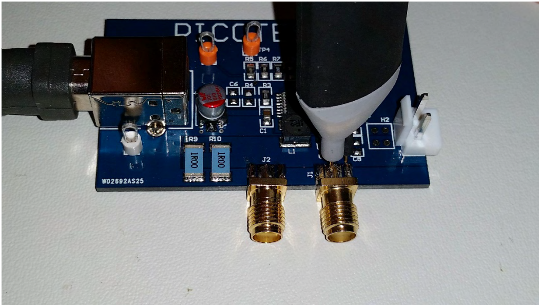
Figure 8: The 1-port probe is terminated into a P2130A DC Blocker and a 50Ohm scope input.
