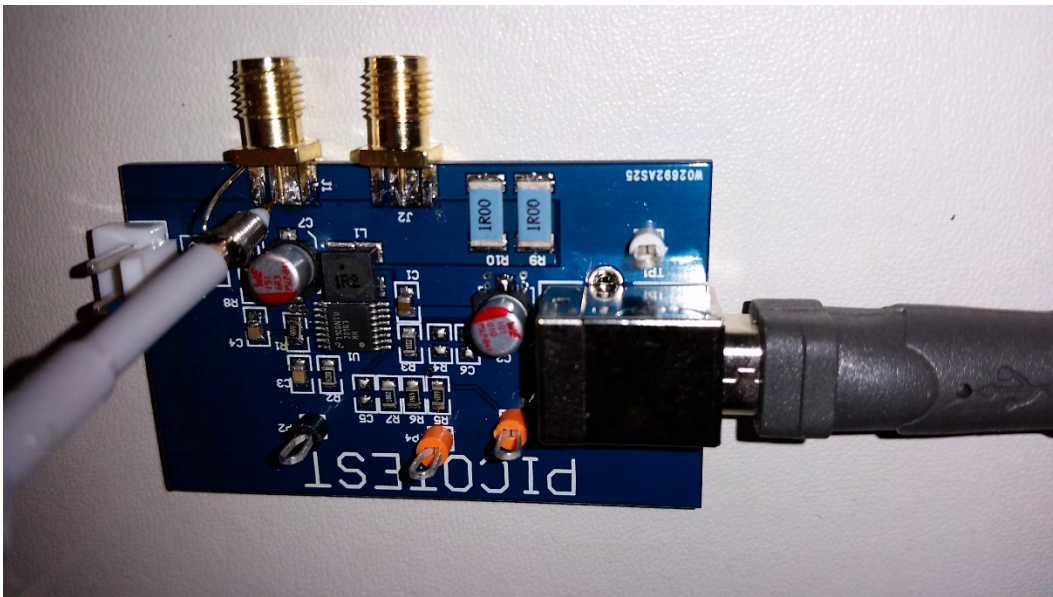
Figure 10: A 10X 500MHz scope probe with short spring clip.
