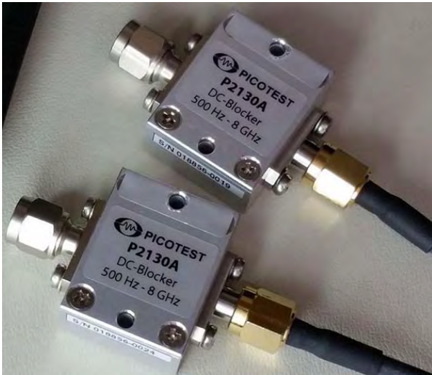
Figure 14: The P2130A DC blocker has a frequency response of 500Hz – 8GHz.
