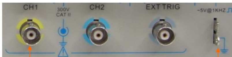
CH1: to connect with the probe
