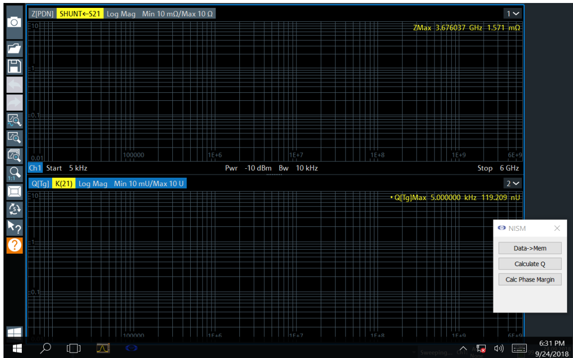
Figure 9: Initialized state of the instrument after running the NISM software. Not the NISM dialog to the right.
