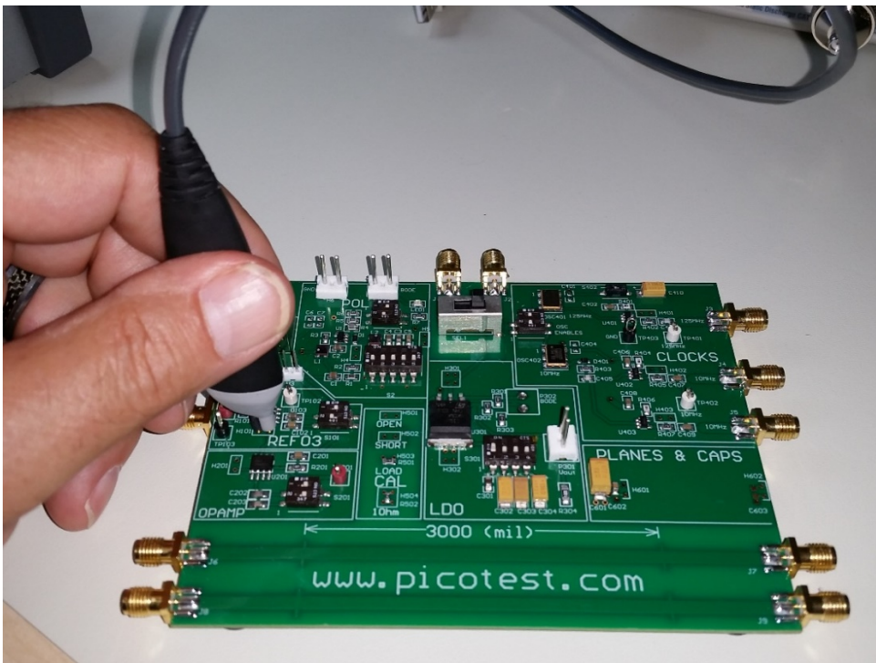
Figure 20: Opamp circuit and H201 test point. The H201 test point can be measured using the Picotest 1 Port PDN probe. The picture above shows the reference being tested. The H201 test point is just below the reference.
