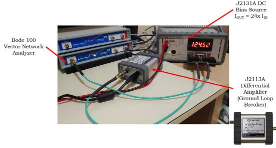
Figure 5: Test Setup Wiring Example with J2113A Differential Amplifier
