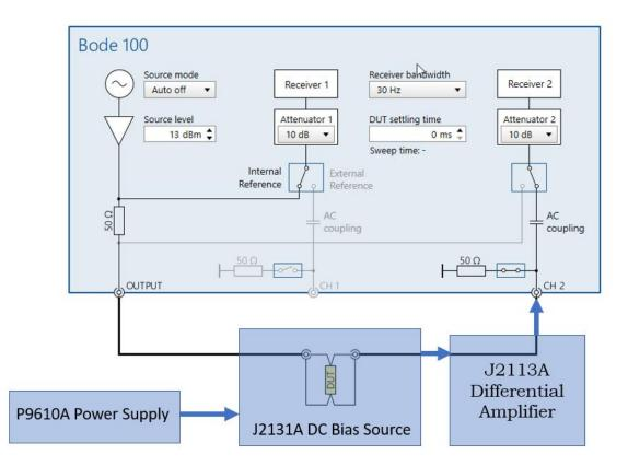
**Figure 6: Test Equipment Configuration**
