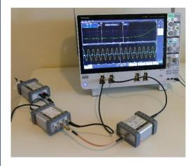
2-Port Shunt-Through test set up using the Tektronix Series 6 osciiloscope, J2161A and J2102B.
