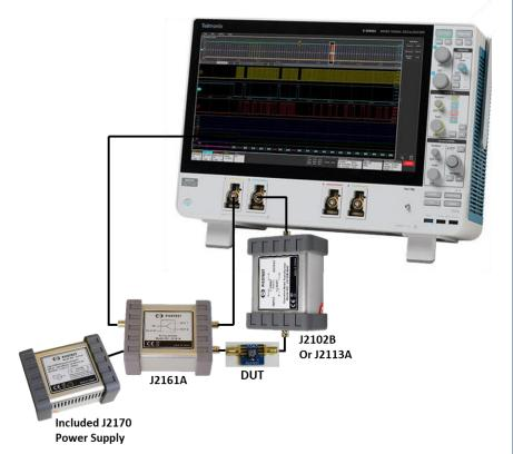
Measurement set up to test ultra-low impedance in the 2-port shunt-through configuration using oscilloscopes and the Picotest J2102B/J2113A ground loop breaker solutions.
