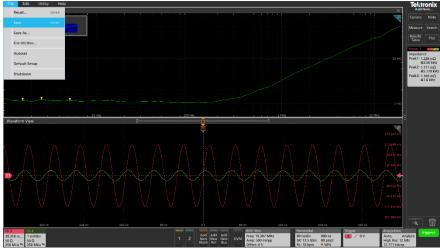
A known 1 m $\Omega$  resistor measured using 2-port shunt-through impedance measurements using the Tektronix Series 6 scope. The J2102B removes the ground loop error in 2-port shunt-through impedance measurements.
