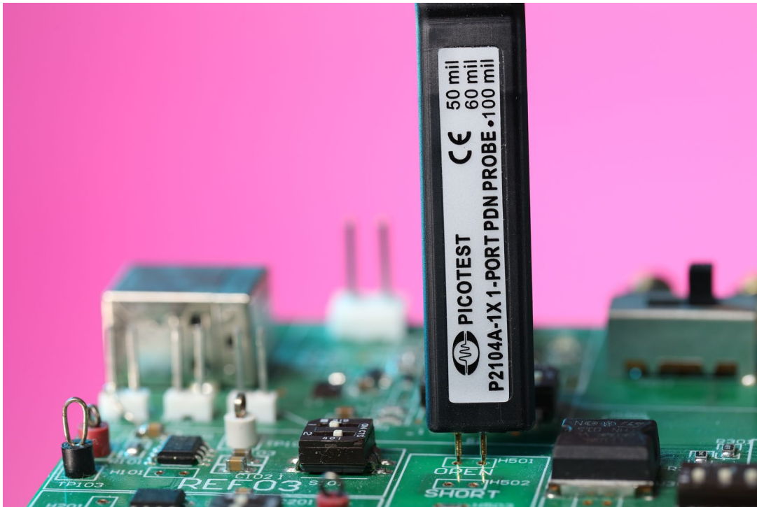
Figure 9: The center pin is the positive pin on the P2104 q-port probe.
