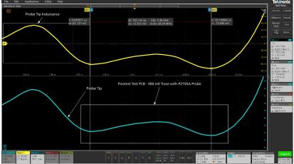
Using the low-cost J2154A, along with the Picotest P2105A TDR probe for injection, you can test PCB coupon impedance. This image shows the change from 47 to 51 Ohms.
