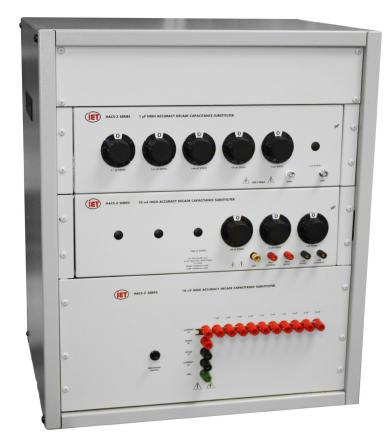
HACS-Z Capacitance Substituter: 9-decade, 10 pF through 1000 μF steps
