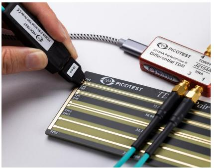
The P2103A TDR probe shown with the Picotest J2154A PerfectPulse<sup>®</sup> Differential TDR makes a powerful and low-cost PCB testing tool. When combined with your oscilloscope, you can probe all types of PCB structures and measure their impedance accurately.
