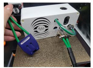
Water cooling technology allows for high power delivery in the custom probe head.
