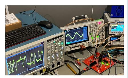
The P2124A enables power supply noise tolerance testing. Here noise is being combined with the power supply input voltage using the P2124A and then onto the DUT board using the near zero interconnect impedance probe head in a QSFP noise immunity test.
