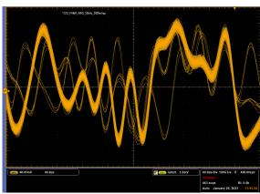
112G PAM4: Noise applied (50kHz), exceeding test level required.
